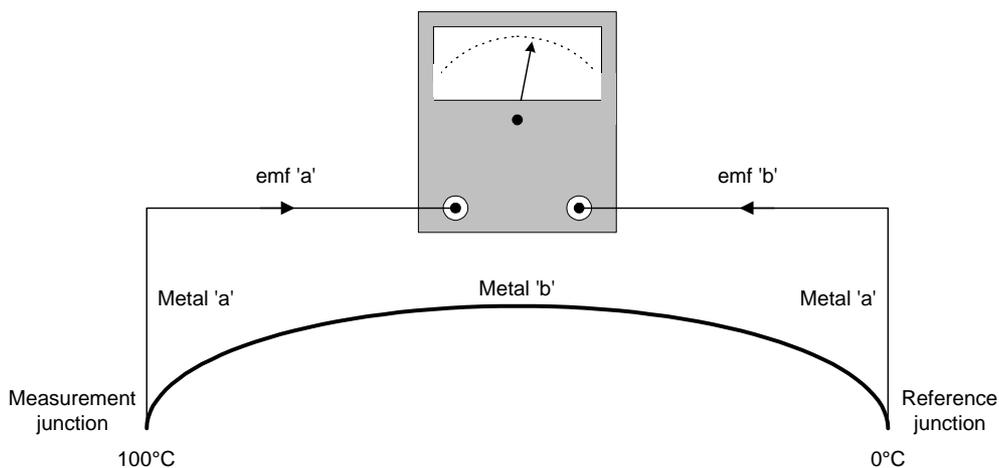
**Figure A.8 Thermocouple principle**
