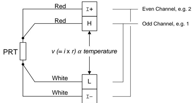
**Figure A.5** Temperature measurement with a PRT
