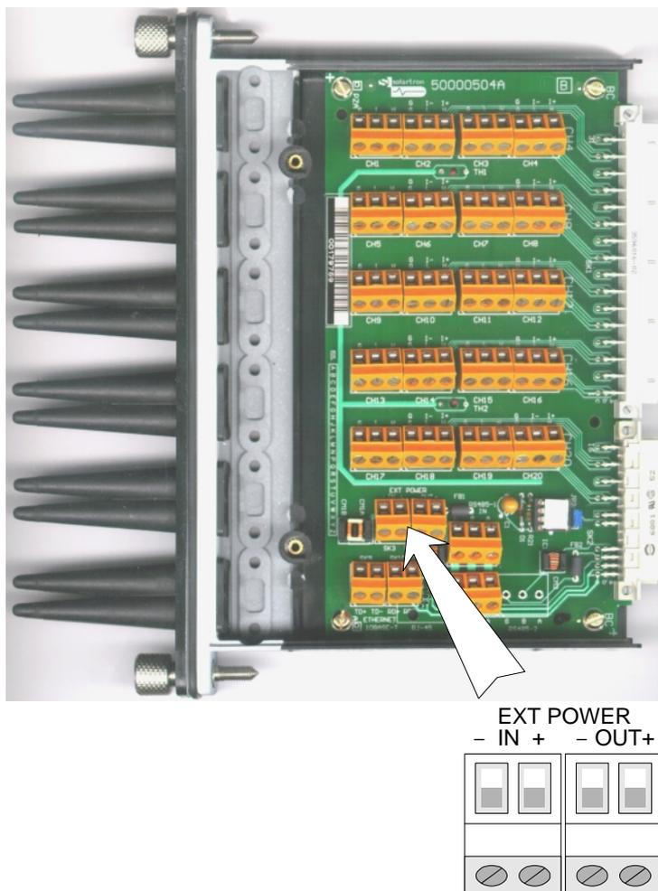
Figure 3.8 External power connectors on the 5000 13L Connector Board.
