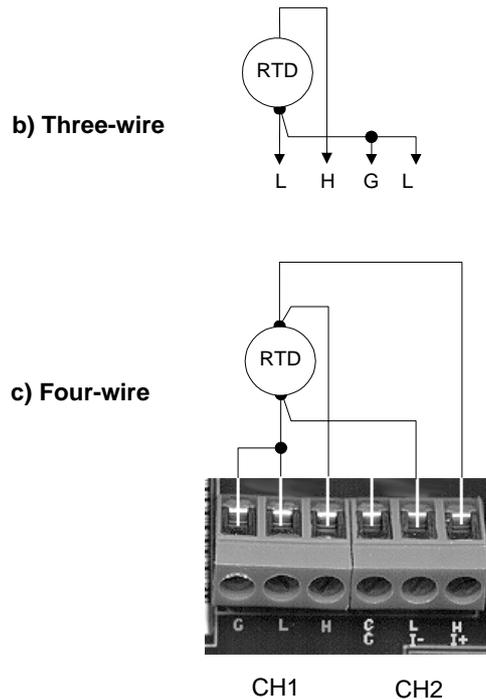
**Figure 4.8 RTD connections.**
