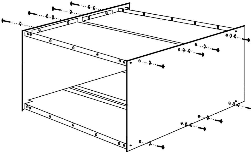
**Figure 3.2** Assembly of support trays and side panels for IMP mounting frame.
