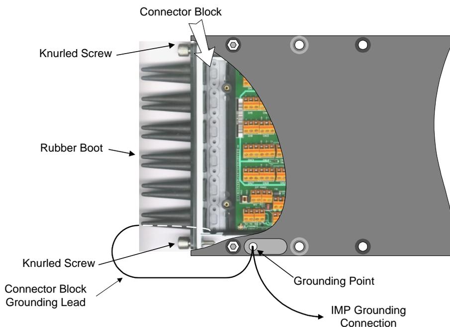
**Figure 3.9** Detail of IMP grounding stud.
