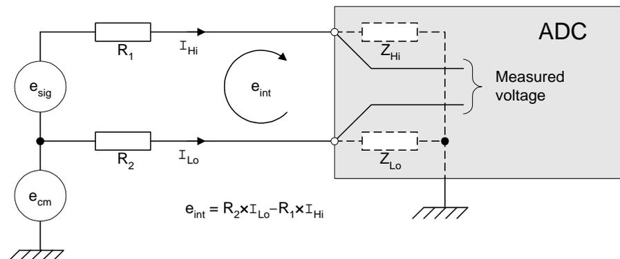
**Figure A.11 Common mode interference**
