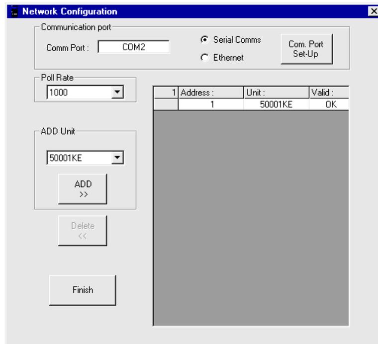
*Initially, a red 'No resp' (no response) indication appears in the Valid column. When the IMP responds to the search this changes to 'OK', which proves that the IMP is set up and responding correctly.*
