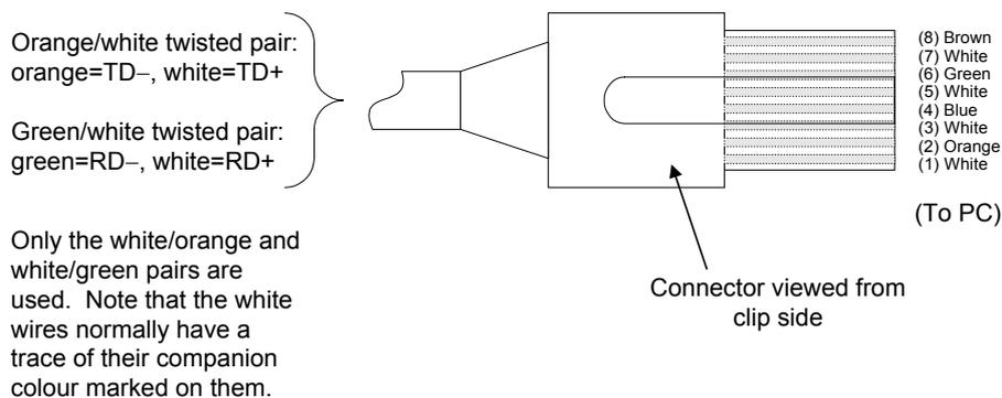
**Figure 2-4 Ethernet cable connections.**
