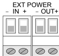
The power source must provide a dc voltage in the range 12V through 24V. The 'IN' and 'OUT' power terminals allow several IMPs to be 'daisy chained' to the supply lines. Connect the power terminals to terminals of the same polarity on the power supply unit. Should you inadvertently reverse the polarity of the supply the IMP will not be damaged –it is reverse polarity protected: to make the IMP work simply switch the polarity over.
