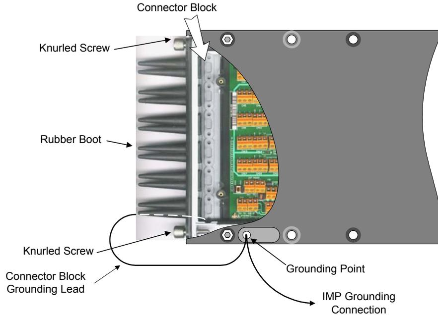
**Figure 2-1** The 5000 13L IMP connector block, inserted into the main IMP housing.
