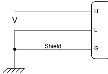
**Figure A.15 Grounded signal guarding**
