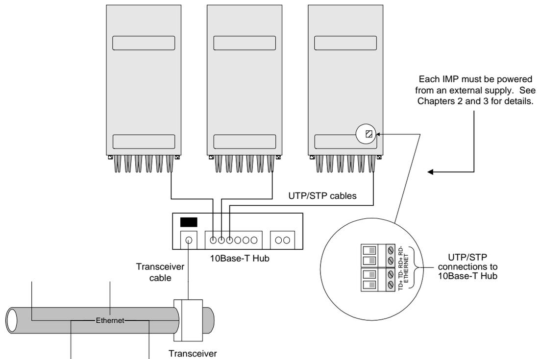
**Figure 5.4 10Base-T network off coax. backbone.**
