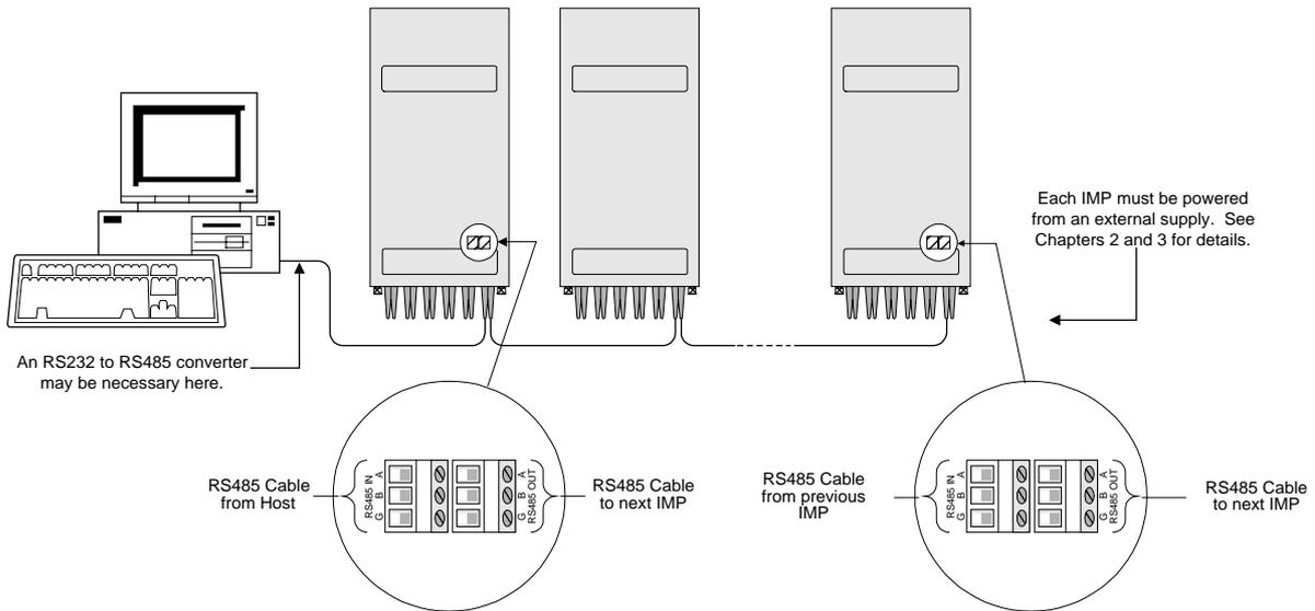
Figure 5.1 RS485 topology for 5000 IMPs.
