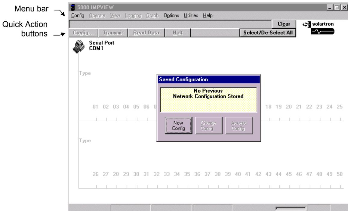
*Initially, the network diagram shows only the PC (serial port). The remainder of the diagram is greyed-out, which indicates that no IMPs have yet been configured: this is reflected by the message in the Saved Configuration window, which tells you that 'No previous network configuration [is] stored'. The only option available at this time is to select **New Configuration**.*
