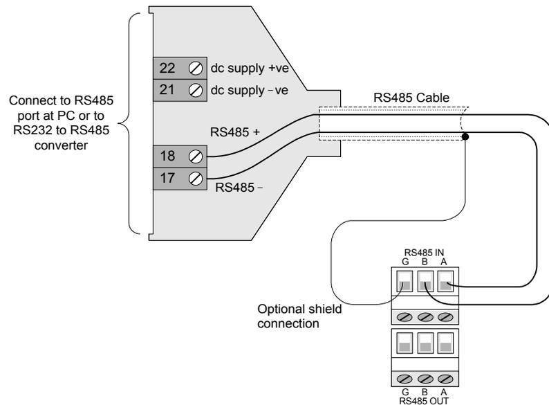
**Figure 2-5 RS485 connections between an IMP and the controlling PC.**
