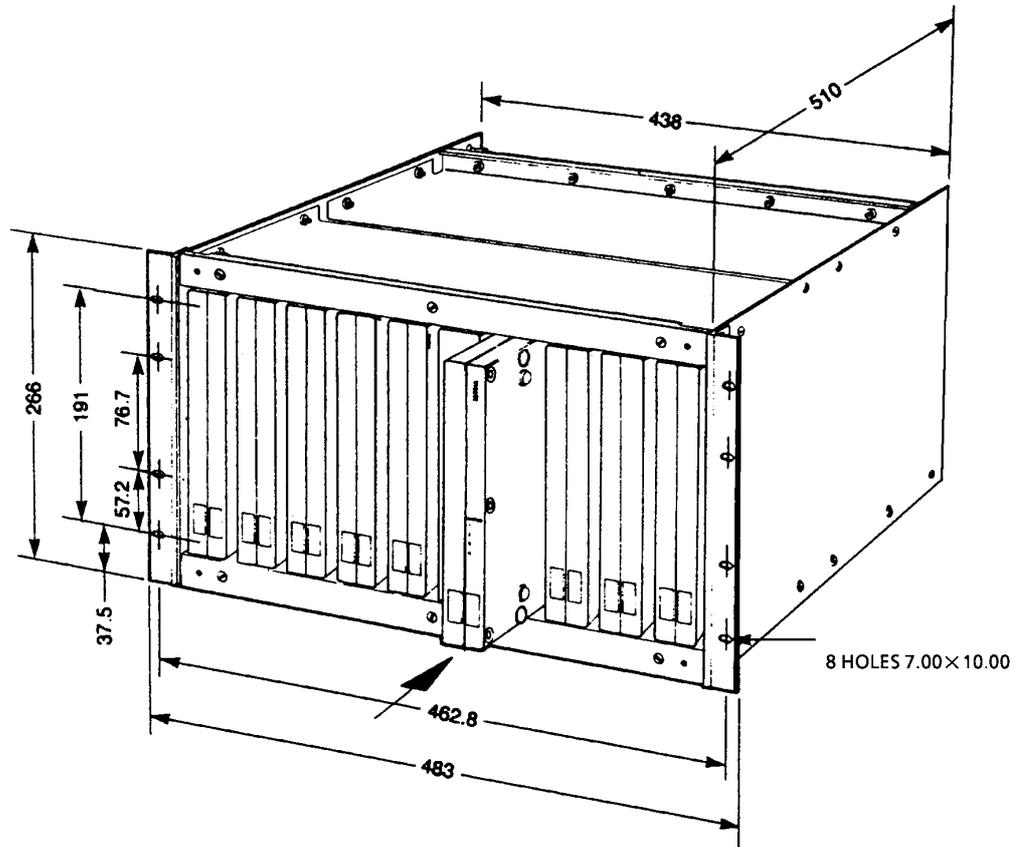
**Figure 3.7** Inserting an IMP into the assembled mounting frame.
