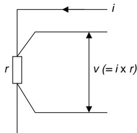
Figure A.2 Principle of resistance measurement
