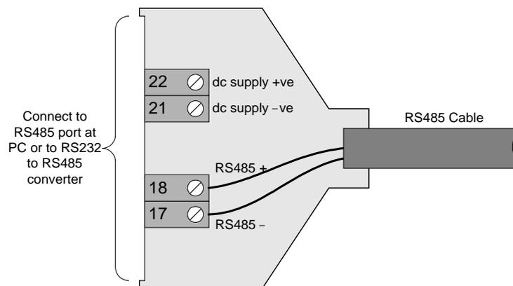
**Figure 5.2 RS485 connections at the Host computer.**
