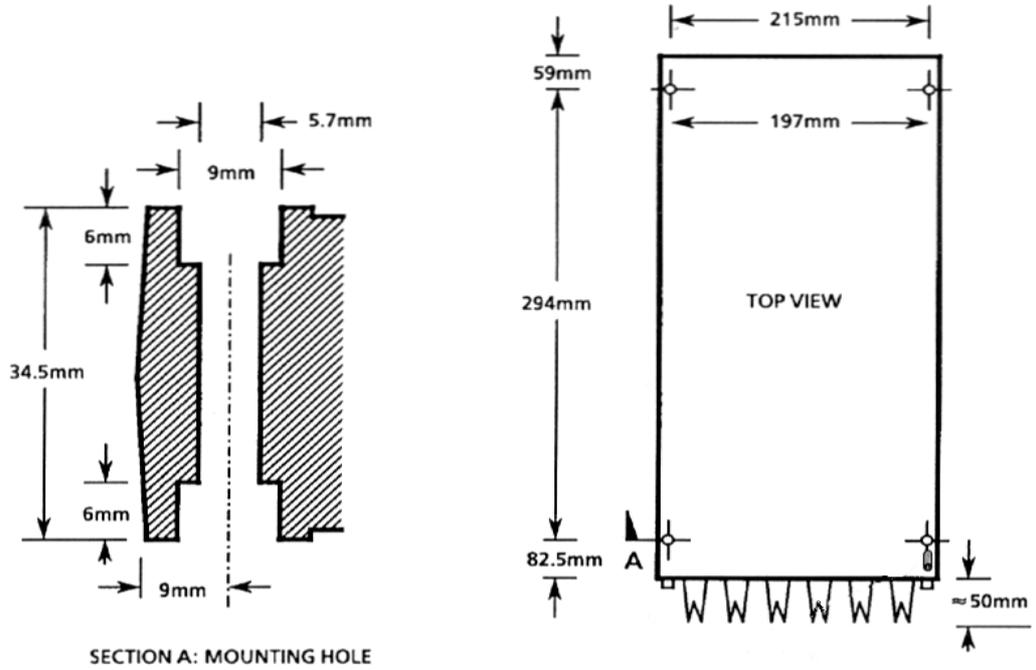
**Figure 3.1** Location of bolt holes on the 5000 IMP.
