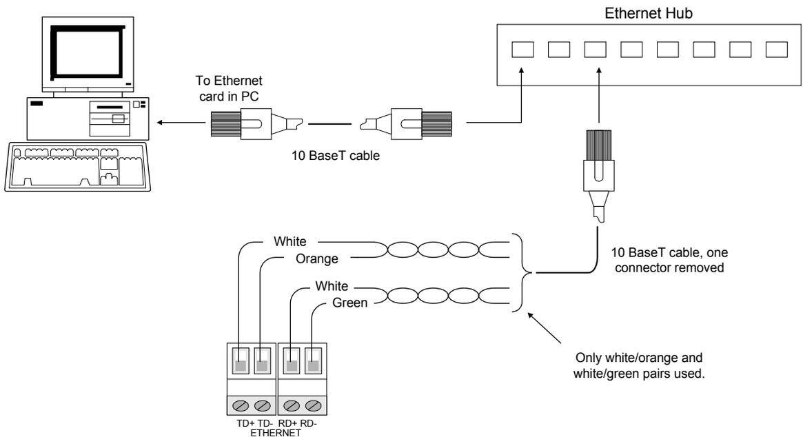
**Figure 2-2** Connecting an IMP to a PC via an Ethernet hub.
