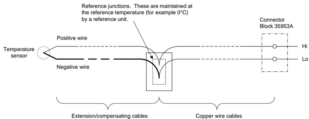
**Figure A.9 Thermocouple connections made through reference unit**
