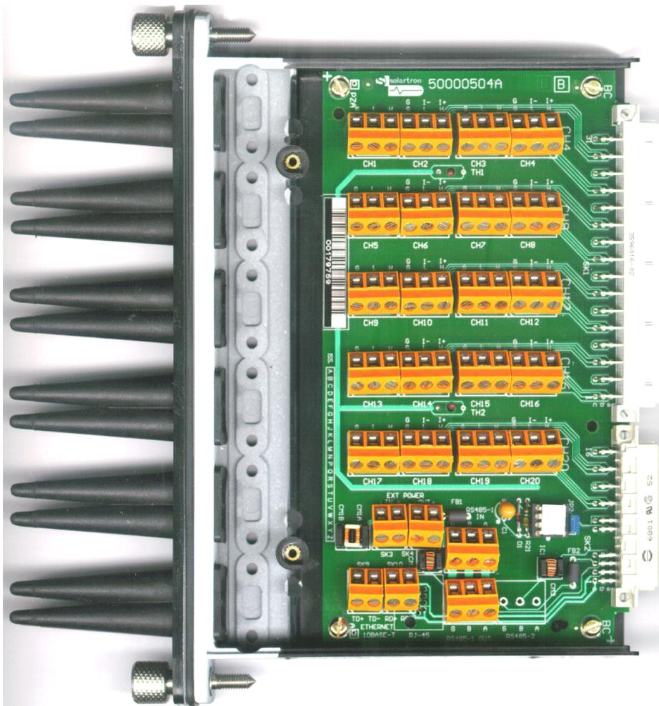
**Figure 4.1** The 5000 13L Connector Block.
