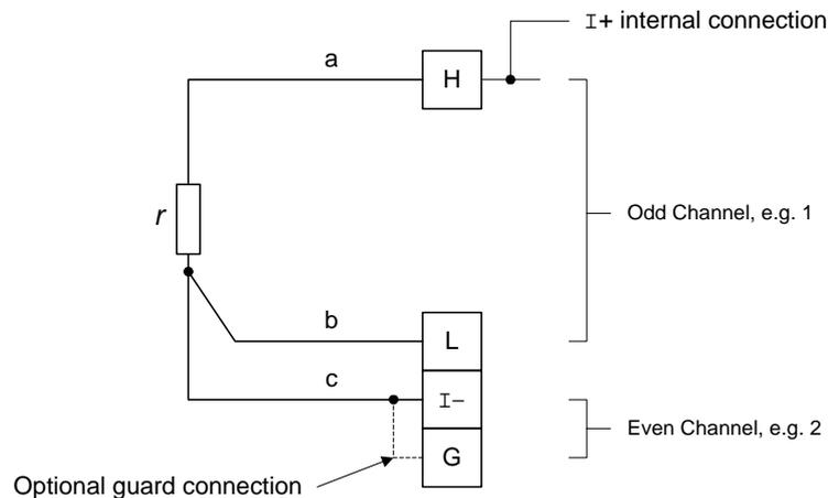
**Figure A.4 Resistance measurement connections, three-wire**
