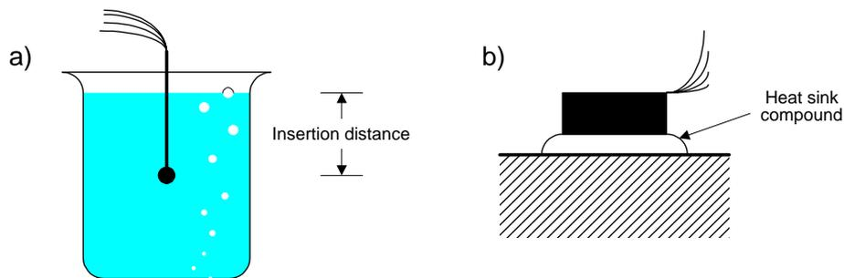
**Figure A.6** Installing a PRT: (a) insertion type; (b) surface mounted type
