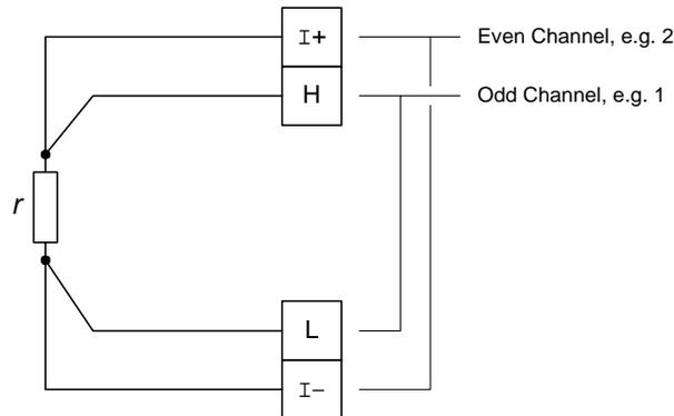
**Figure A.3 Resistance measurement connections, four-wire**
