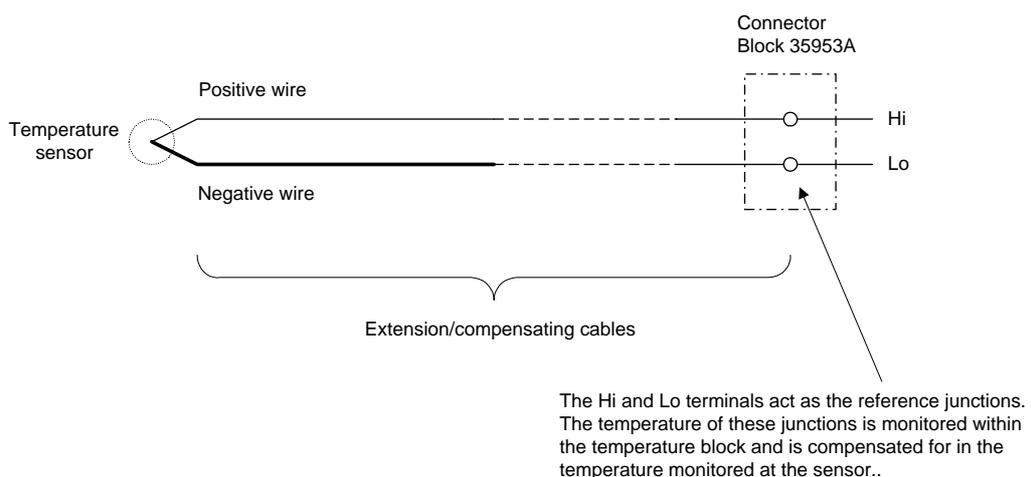
**Figure A.10 Thermocouple connections made direct to the connector block**
