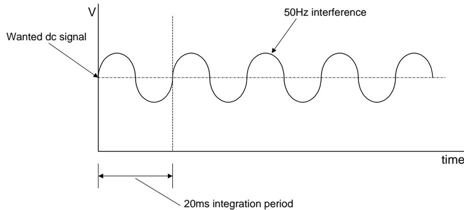
**Figure A.13** The rejection of ac series mode interference at 50 Hz
