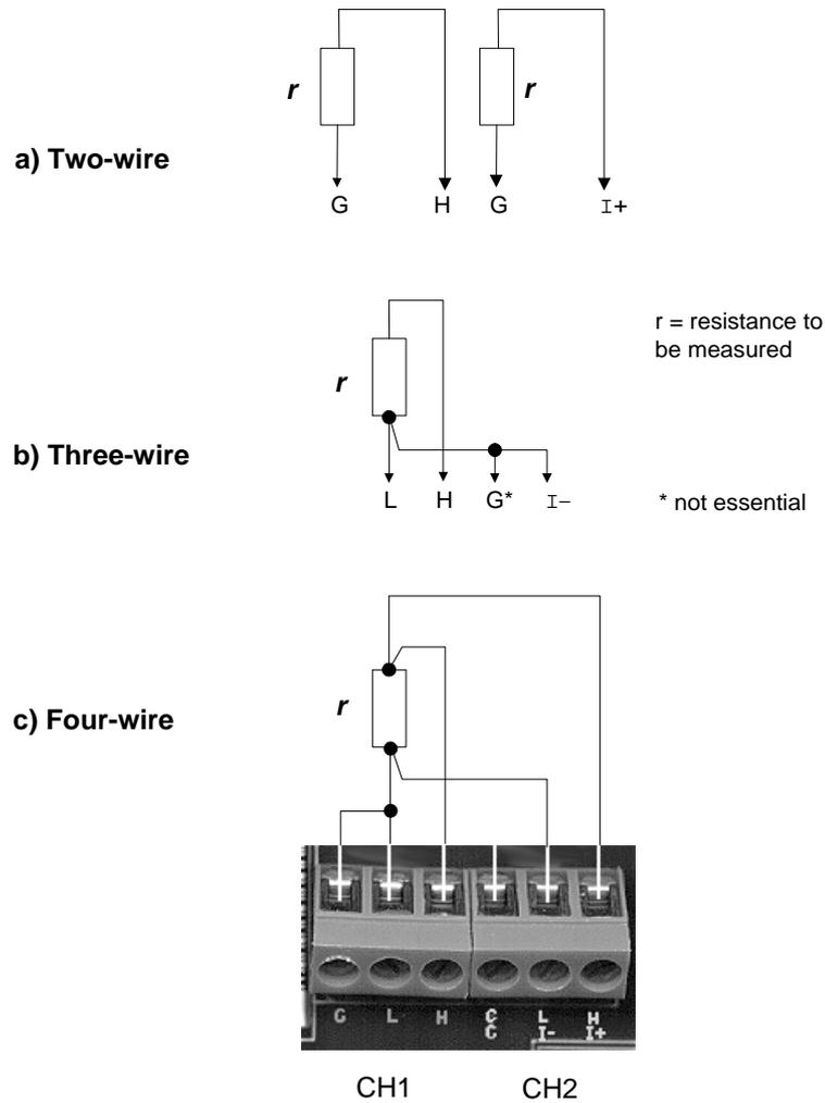
Figure 4.6 Resistance connections.
