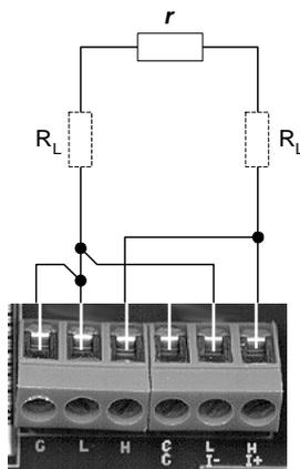
Figure 4.7 Four-wire connections for two-wire source.
