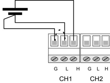
**Figure 2-6 Example of measurement channel connections.**
