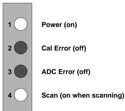
**Figure 4.11** Normal state of LED status indicators.
