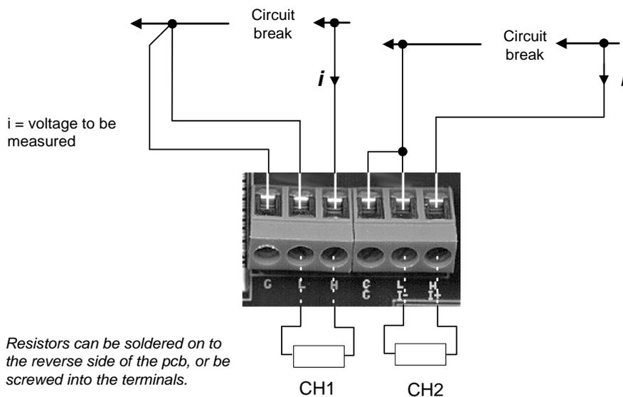
**Figure 4.4 Example of current connections.**
