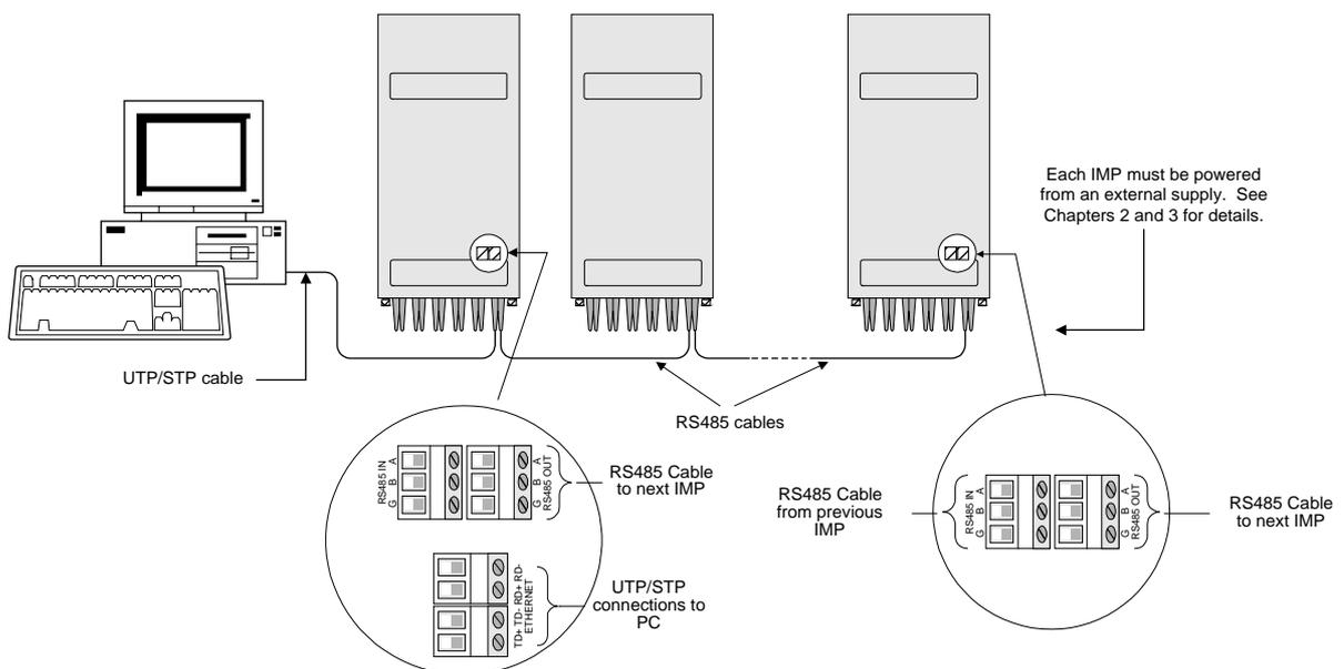
**Figure 5.5** Pass-through control connections.
