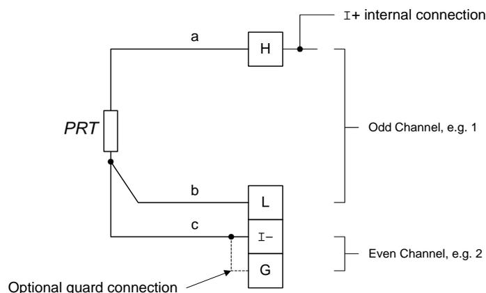
**Figure A.7** PRT connections, three-wire method
