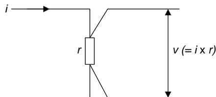
Figure A.1 Principle of current measurement
