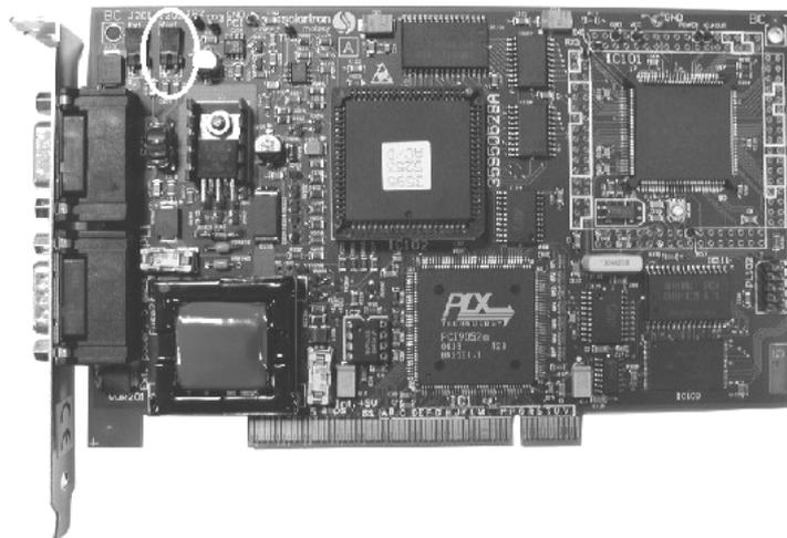
Figure 2.2: Location of S-Net termination Jumper J202
