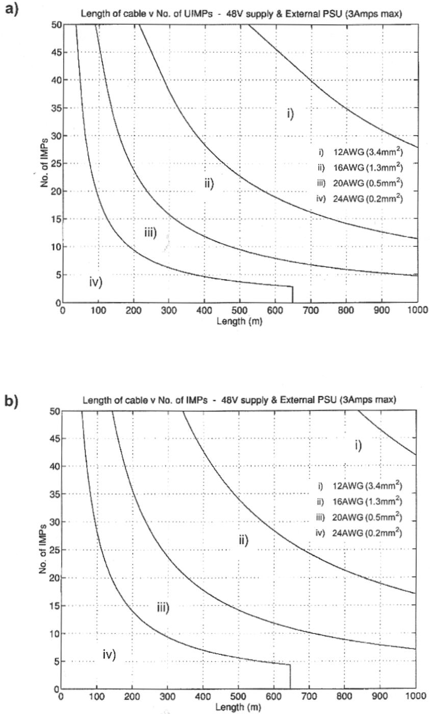
Figure 2.8: Minimum recommended wire gauge for a 48V external supply for:
