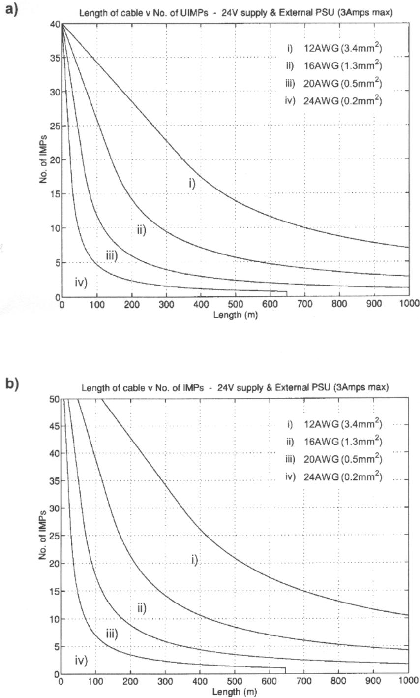
Figure 2.7: Minimum recommended wire gauge for a 24V external supply for:
