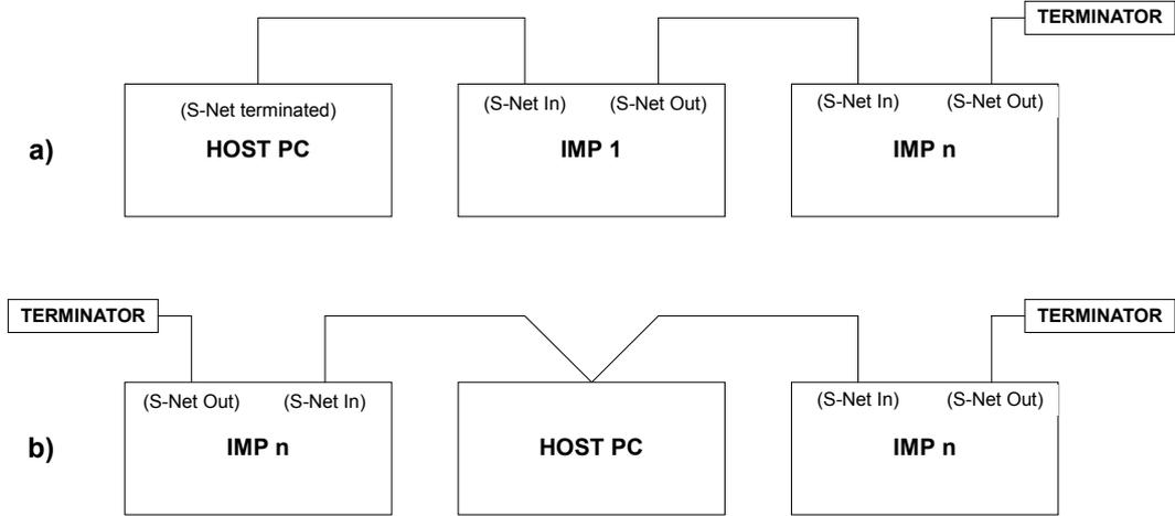
Figure 2.1: S-Net cable terminations
