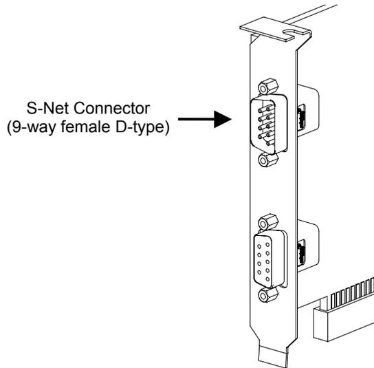
Figure 2.6: Location of S-Net connector on the Host PC rear panel
