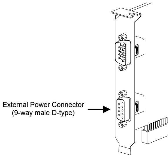
Figure 2.9: Location of the external power connector on the PC rear panel
