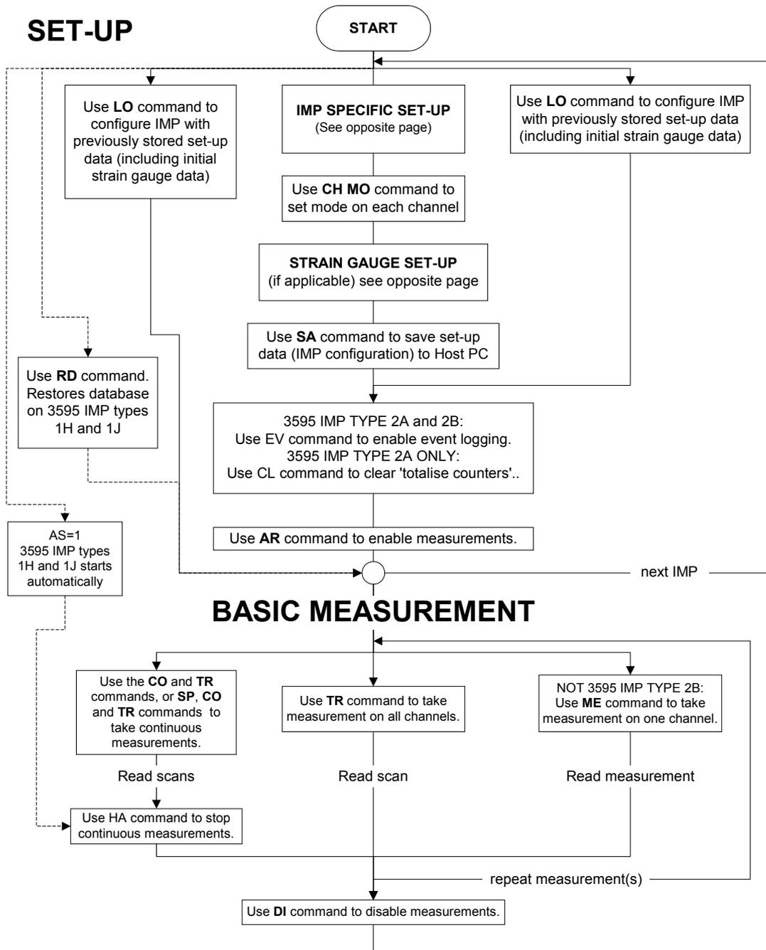
Figure 1.5: Set-up and basic measurement
