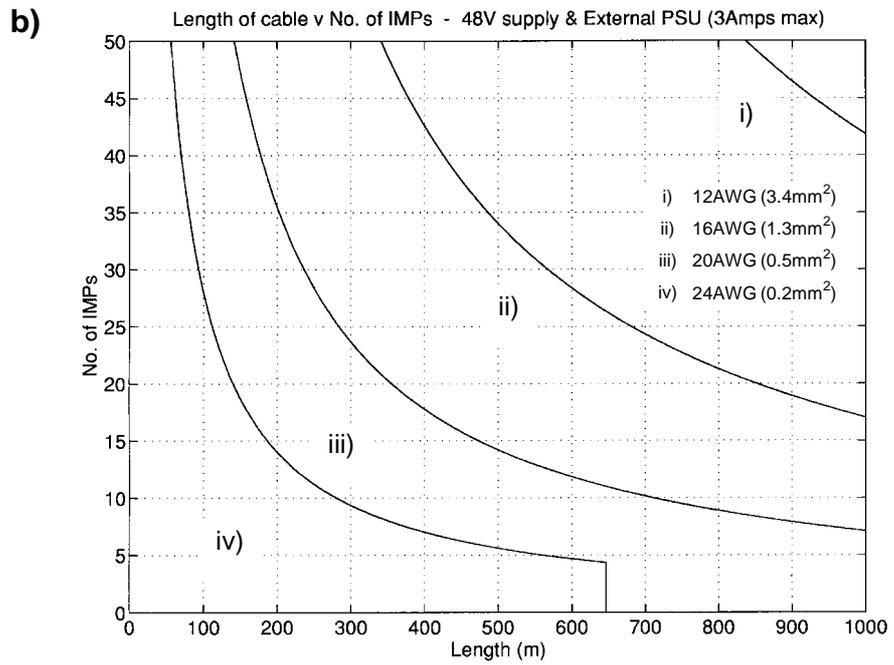
**Figure 2.16** Minimum recommended wire gage for a 48V external supply for:
