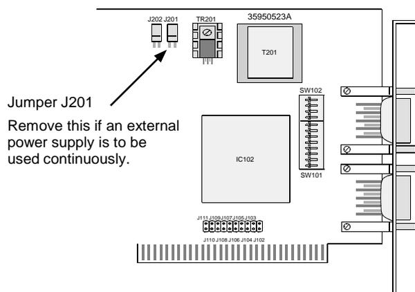
**Figure 2.11** Location of the external supply jumper J201
