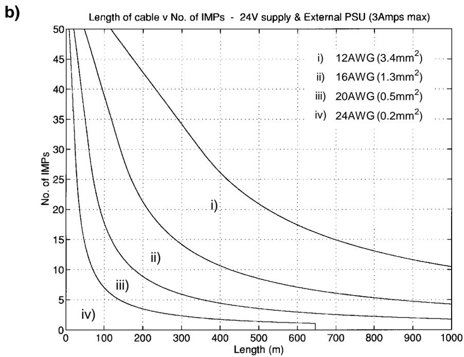
**Figure 2.15** Minimum recommended wire gage for a 24V external supply for:
