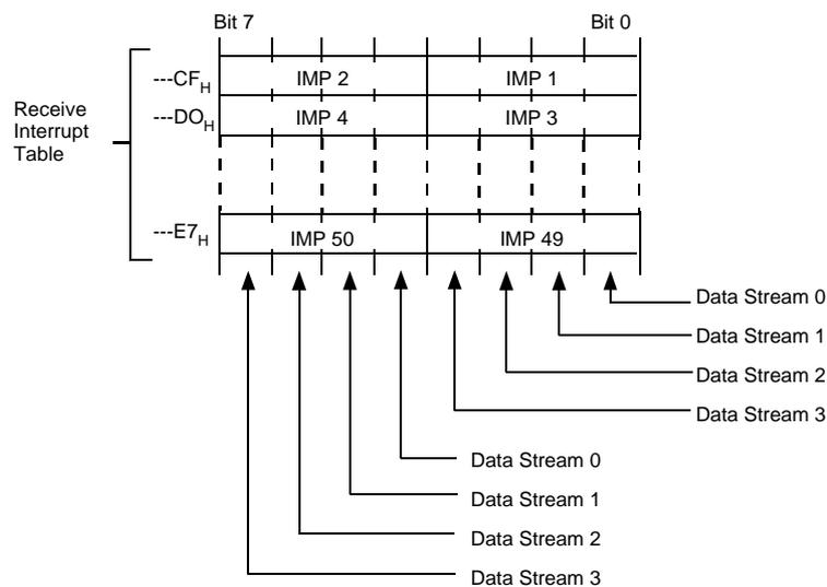
**Figure 4.8 Receive interrupt table.**
