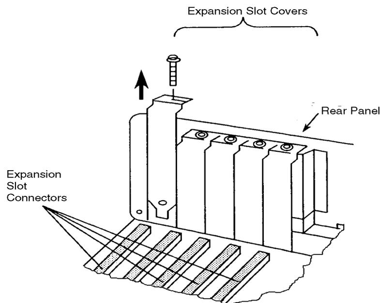
**Figure 2.12** Removal of expansion slot cover.
