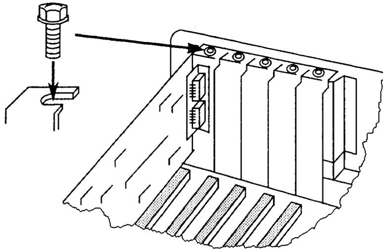
**Figure 2.13 Fitting the interface card retaining screw.**
