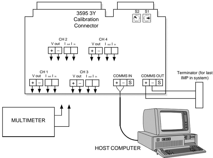
**Figure 1.2 Connections to 3595 3Y calibration connector block.**
