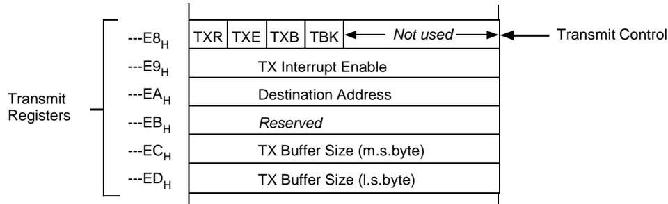
**Figure 4.6 Transmit registers.**
