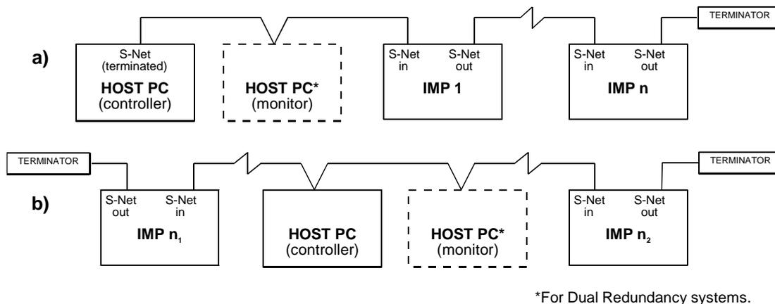
**Figure 2.1 S-Net cable terminations**
